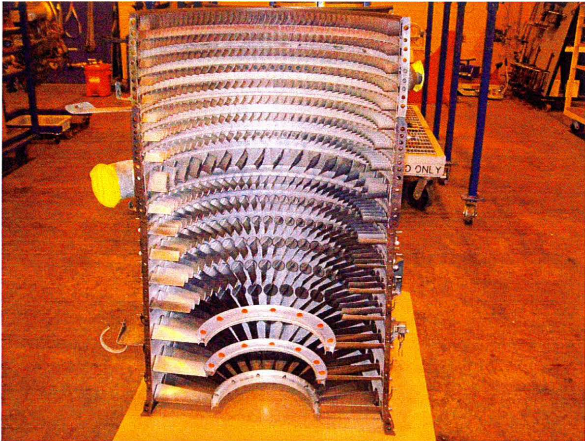
UPPER COMPRESSOR CASE AFTER REMOVAL
